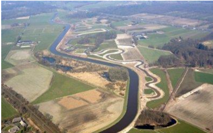
A De Dommel water board project shows how reclaimed land polders are being given back to rivers and meanders are cut into flood plains, as part of Netherland's back-to-nature approach. Photograph: Courtesy De Dommel Waterboard
