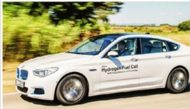
A BMW 5-Series Gran Turismo hydrogen fuel-cell prototype car
