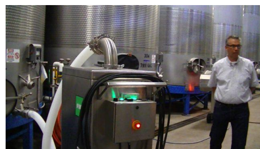
This unit sends fog into the fermentation tanks to clean them before they are filled with a new batch of wine.
