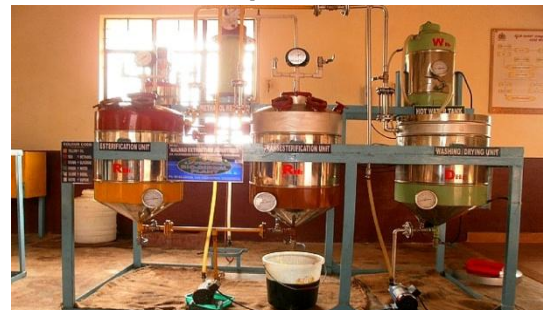
The setup for the process of converting used cooking oil to biodiesel
