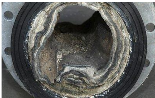
A cross-section of pipe from a Thames Water sewage works in which struvite, a nutrient compound containing phosphorous, has built up. If left unchecked, struvite blocks these pipes completely Photograph: Stewart Turkington/Thames Water
