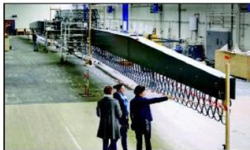
GOING GREEN: The 72-metre-long wing of Swiss sun-powered aircraft Solar Impulse HB-SIB is made of carbon fibre
